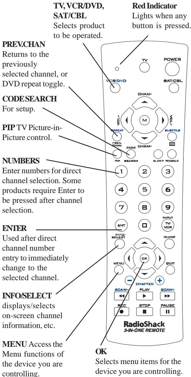
Note: The **REC** button must be pressed **TWICE** to record from your VCR. For some brands of VCRs, you might need to press the **REC** button once, and then press it again for three seconds.
