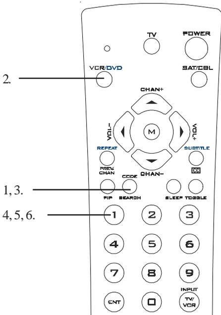
The Sleep button accesses the sleep function of your TV if it has that feature. If it does not, you can enable the remote to turn off your TV after a period of 1 to 99 minutes, as shown below. The remote must be in TV mode to set a Sleep Timer. This feature works even if your TV does not have a sleep feature.
